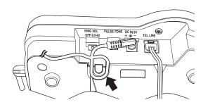
5. Plug the other end of the telephone cord into the telephone jack on the wall.
